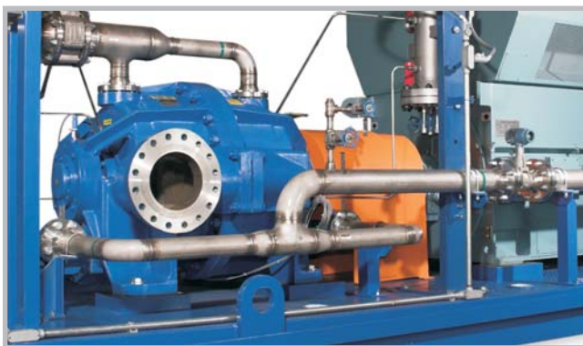
NASH HP-9 Flare Gas Recovery Unit
